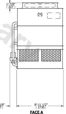
DRAWN BY: SLR NO. OF SHIPPING SECTIONS **SHIPPING** OPERATING HEAVIEST SECTION 9150 lbs+ [4155] kg+ 10590 lbs+ [4805] kg+ 13700 lbs+ [6215] kg+ WEIGHT WEIGHT WEIGHT
