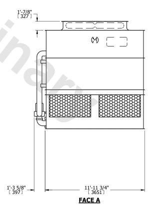
DRAWN BY: SLR NO. OF SHIPPING SECTIONS **SHIPPING** OPERATING HEAVIEST SECTION 13230 lbs+ [6005] kg+ 11430 lbs+ [5185] kg+ 17530 lbs+ [7955] kg+ WEIGHT WEIGHT WEIGHT
