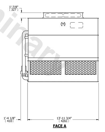
DRAWN BY: SLR NO. OF SHIPPING SECTIONS **SHIPPING** OPERATING HEAVIEST SECTION 17070 lbs+ [7745] kg+ 15060 lbs+ [6835] kg+ 22210 lbs+ [10075] kg+ WEIGHT WEIGHT WEIGHT
