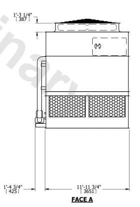
SHIPPING WEIGHT 18800 lbs+ [8530] kg+ OPERATING WEIGHT 25780 lbs+ [11695] kg+ HEAVIEST SECTION WEIGHT 16090 lbs+ [7300] kg+ NO. OF SHIPPING SECTIONS 2 DRAWN BY: SLR
