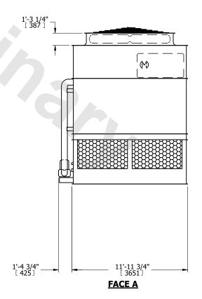
NO. OF SHIPPING SECTIONS **SHIPPING** OPERATING HEAVIEST SECTION 21400 lbs+ [9710] kg+ 18690 lbs+ [8480] kg+ 28560 lbs+ [12955] kg+ WEIGHT WEIGHT WEIGHT
