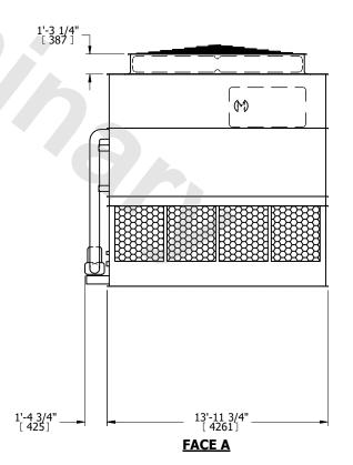
DRAWN BY: NO. OF SHIPPING SECTIONS **SHIPPING** OPERATING HEAVIEST SECTION 18940 lbs+ [8595] kg+ 15880 lbs+ [7205] kg+ 26940 lbs+ [12220] kg+ WEIGHT WEIGHT WEIGHT
