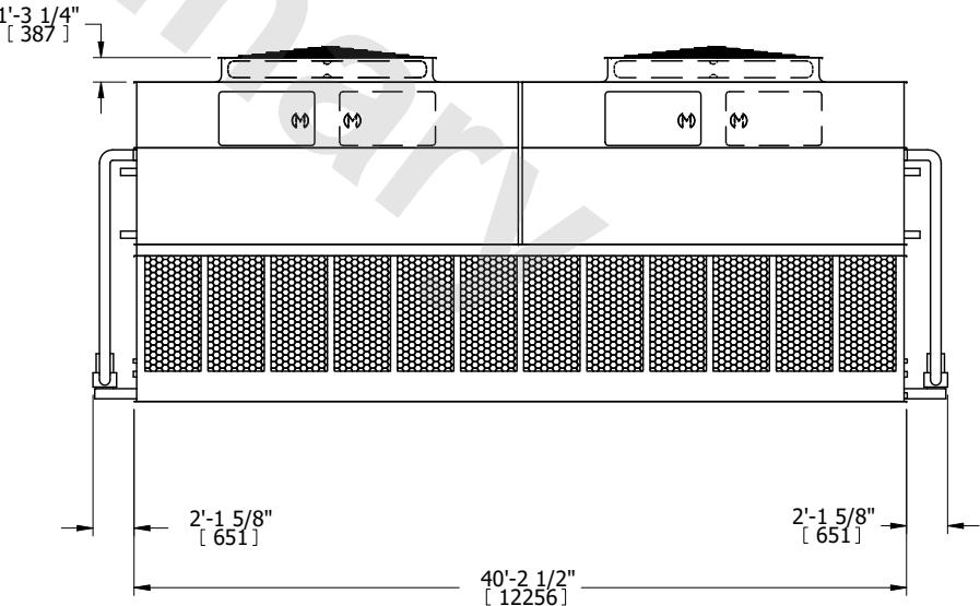
SHIPPING WEIGHT 120260 lbs+ [54550] kg+ OPERATING WEIGHT 167600 lbs+ [76025] kg+ HEAVIEST SECTION WEIGHT 25530 lbs+ [11585] kg+ NO. OF SHIPPING SECTIONS 6 DRAWN BY: SLR
