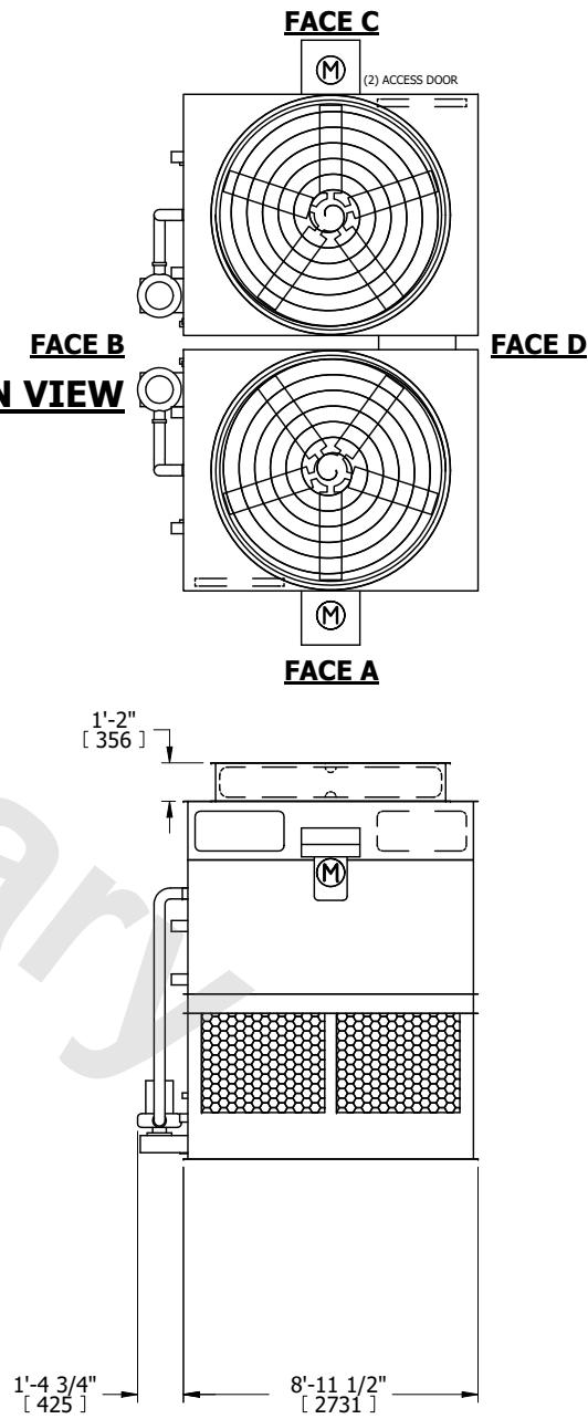
SHIPPING WEIGHT 22500 lbs+ [10210] kg+ OPERATING WEIGHT 24060 lbs+ [10915] kg+ HEAVIEST SECTION WEIGHT 8200 lbs+ [3720] kg+ NO. OF SHIPPING SECTIONS 4 DRAWN BY: TAM
