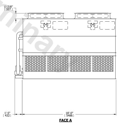
SHIPPING WEIGHT 16830 lbs+ [7635] kg+ OPERATING WEIGHT 22360 lbs+ [10145] kg+ HEAVIEST SECTION WEIGHT 14100 lbs+ [6400] kg+ NO. OF SHIPPING SECTIONS 2 DRAWN BY: SLR
