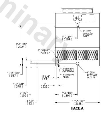
SHIPPING WEIGHT 5470 lbs+ [2485] kg+ OPERATING WEIGHT 8770 lbs+ [3980] kg+ HEAVIEST SECTION WEIGHT 3870 lbs+ [1760] kg+ NO. OF SHIPPING SECTIONS 2 DRAWN BY: JLG
