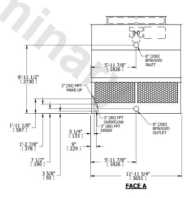
SHIPPING WEIGHT 5660 lbs+ [2570] kg+ OPERATING WEIGHT 9520 lbs+ [4320] kg+ HEAVIEST SECTION WEIGHT 3900 lbs+ [1770] kg+ NO. OF SHIPPING SECTIONS 2 DRAWN BY: JLG
