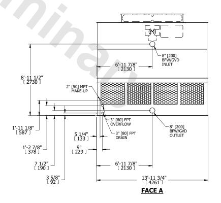
SHIPPING WEIGHT 6310 lbs+ [2865] kg+ OPERATING WEIGHT 10820 lbs+ [4910] kg+ HEAVIEST SECTION WEIGHT
