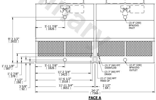
DRAWN BY: JLG SHIPPING WEIGHT OPERATING WEIGHT HEAVIEST SECTION WEIGHT NO. OF SHIPPING SECTIONS 3820 lbs+ [1735] kg+ 11360 lbs+ [5155] kg+ 19080 lbs+ [8655] kg+
