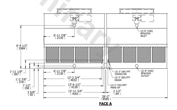
SHIPPING WEIGHT 12760 lbs+ [5790] kg+ OPERATING WEIGHT 21780 lbs+ [9880] kg+ HEAVIEST SECTION WEIGHT 4240 lbs+ [1925] kg+ NO. OF SHIPPING SECTIONS 4 DRAWN BY: JLG
