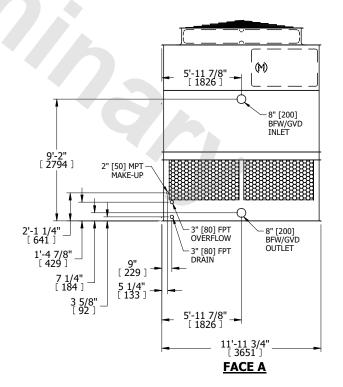
DRAWN BY: KDS NO. OF SHIPPING SECTIONS **SHIPPING** OPERATING HEAVIEST SECTION 8040 lbs+ [3650] kg+ 14250 lbs+ [6465] kg+ 5640 lbs+ [2560] kg+ WEIGHT WEIGHT WEIGHT
