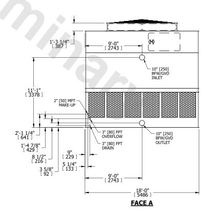
DRAWN BY: KDS SHIPPING NO. OF SHIPPING SECTIONS OPERATING HEAVIEST SECTION 12600 lbs+ [5720] kg+ 21870 lbs+ [9925] kg+ 8700 lbs+ [3950] kg+ WEIGHT WEIGHT WEIGHT
