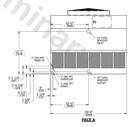
SHIPPING WEIGHT 13370 lbs+ [6065] kg+ OPERATING WEIGHT 23770 lbs+ [10785] kg+ HEAVIEST SECTION WEIGHT 9260 lbs+ [4205] kg+ NO. OF SHIPPING SECTIONS 2 DRAWN BY: KDS
