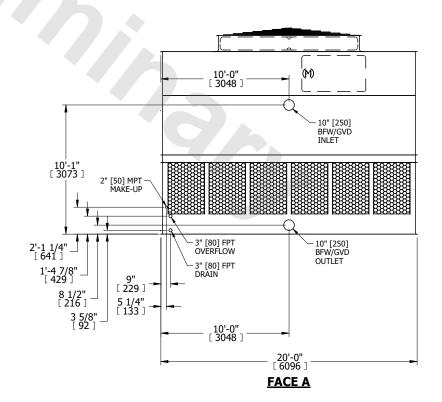
DRAWN BY: KDS NO. OF SHIPPING SECTIONS **SHIPPING** OPERATING HEAVIEST SECTION 12530 lbs+ [5685] kg+ 22930 lbs+ [10405] kg+ 8420 lbs+ [3820] kg+ WEIGHT WEIGHT WEIGHT
