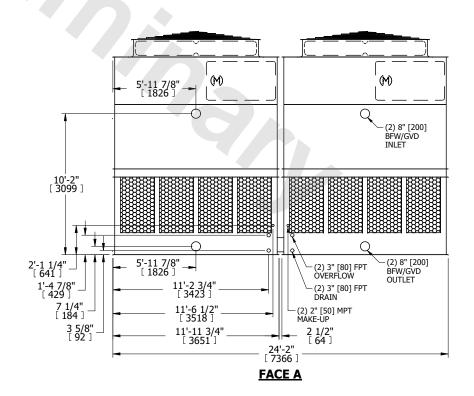
SHIPPING WEIGHT 16160 lbs+ [7335] kg+ OPERATING WEIGHT 28580 lbs+ [12965] kg+ HEAVIEST SECTION WEIGHT 5540 lbs+ [2515] kg+ NO. OF SHIPPING SECTIONS 4 DRAWN BY: KDS
