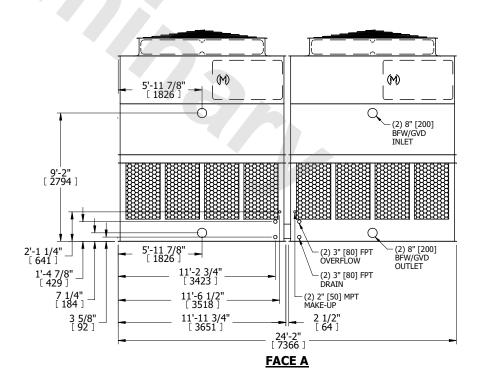
SHIPPING WEIGHT 15480 lbs+ [7025] kg+ OPERATING WEIGHT 27900 lbs+ [12660] kg+ HEAVIEST SECTION WEIGHT 5200 lbs+ [2360] kg+ NO. OF SHIPPING SECTIONS 4 DRAWN BY: KDS
