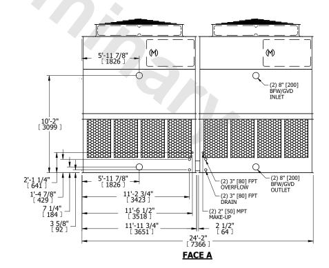
SHIPPING WEIGHT 16360 lbs+ [7425] kg+ OPERATING WEIGHT 28780 lbs+ [13055] kg+ HEAVIEST SECTION WEIGHT 5640 lbs+ [2560] kg+ NO. OF SHIPPING SECTIONS 4 DRAWN BY: KDS
