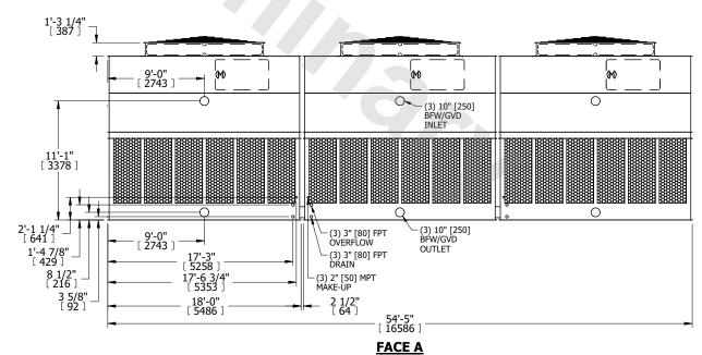
DRAWN BY: KDS NO. OF SHIPPING SECTIONS **SHIPPING** OPERATING HEAVIEST SECTION 33300 lbs+ [15105] kg+ 6920 lbs+ [3140] kg+ 61110 lbs+ [27720] kg+ WEIGHT WEIGHT WEIGHT
