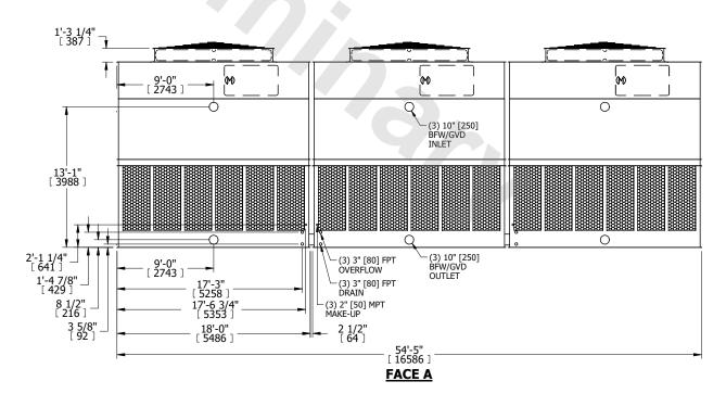
DRAWN BY: KDS NO. OF SHIPPING SECTIONS **SHIPPING** OPERATING HEAVIEST SECTION 37860 lbs+ [17175] kg+ 65670 lbs+ [29790] kg+ 8440 lbs+ [3830] kg+ WEIGHT WEIGHT WEIGHT
