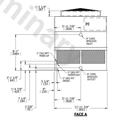
SHIPPING WEIGHT 6890 lbs+ [3130] kg+ OPERATING WEIGHT 11850 lbs+ [5380] kg+ HEAVIEST SECTION WEIGHT 4470 lbs+ [2030] kg+ NO. OF SHIPPING SECTIONS 2 DRAWN BY: JLG
