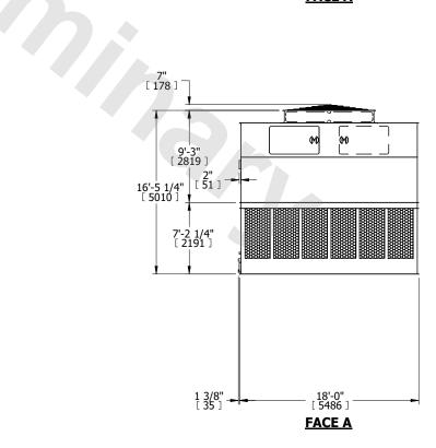
SHIPPING WEIGHT 20820 lbs+ [9445] kg+ OPERATING WEIGHT 36020 lbs+ [16340] kg+ HEAVIEST SECTION WEIGHT 6500 lbs+ [2950] kg+ NO. OF SHIPPING SECTIONS 4 DRAWN BY: JLG
