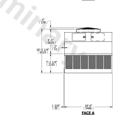
SHIPPING WEIGHT 21520 lbs+ [9765] kg+ OPERATING WEIGHT 36720 lbs+ [16660] kg+ HEAVIEST SECTION WEIGHT 6850 lbs+ [3110] kg+ NO. OF SHIPPING SECTIONS 4 DRAWN BY:
