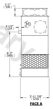
DRAWN BY: KWC NO. OF SHIPPING SECTIONS **SHIPPING** OPERATING HEAVIEST SECTION 1080 lbs+ [490] kg+ 1710 lbs+ [780] kg+ 730 lbs+ [335] kg+ WEIGHT WEIGHT WEIGHT
