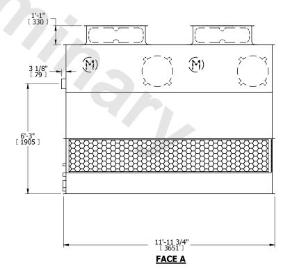
SHIPPING WEIGHT 2570 lbs+ [1170] kg+ OPERATING WEIGHT 4690 lbs+ [2130] kg+ HEAVIEST SECTION WEIGHT 1810 lbs+ [825] kg+ NO. OF SHIPPING SECTIONS 2 DRAWN BY: KWC
