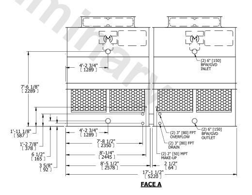
SHIPPING WEIGHT 6400 lbs+ [2905] kg+ OPERATING WEIGHT 10480 lbs+ [4755] kg+ HEAVIEST SECTION 2050 lbs+ [930] kg+ NO. OF SHIPPING SECTIONS 4 DRAWN BY: JLG
