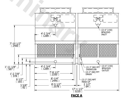
SHIPPING WEIGHT 7260 lbs+ [3295] kg+ OPERATING WEIGHT 12100 lbs+ [5490] kg+ HEAVIEST SECTION WEIGHT 2320 lbs+ [1055] kg+ NO. OF SHIPPING SECTIONS 4 DRAWN BY: JLG
