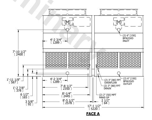
SHIPPING WEIGHT 7320 lbs+ [3325] kg+ OPERATING WEIGHT 12160 lbs+ [5520] kg+ HEAVIEST SECTION WEIGHT 2350 lbs+ [1070] kg+ NO. OF SHIPPING SECTIONS 4 DRAWN BY: JLG
