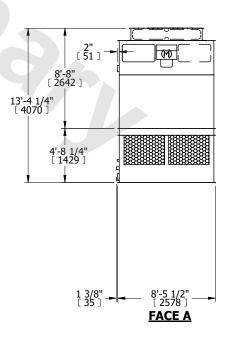
SHIPPING WEIGHT 8380 lbs+ [3805] kg+ OPERATING WEIGHT 13220 lbs+ [6000] kg+ HEAVIEST SECTION WEIGHT 2850 lbs+ [1295] kg+ NO. OF SHIPPING SECTIONS
