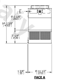
SHIPPING WEIGHT 9960 lbs+ [4520] kg+ OPERATING WEIGHT 15640 lbs+ [7095] kg+ HEAVIEST SECTION WEIGHT 3440 lbs+ [1565] kg+ NO. OF SHIPPING SECTIONS 4 DRAWN BY: KDS
