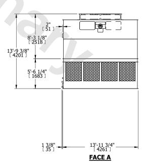
NO. OF SHIPPING SECTIONS **SHIPPING** OPERATING HEAVIEST SECTION 12680 lbs+ [5755] kg+ 4200 lbs+ [1910] kg+ 21700 lbs+ [9845] kg+ WEIGHT WEIGHT WEIGHT
