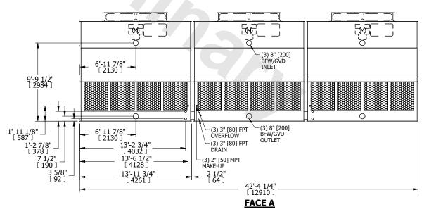
HEAVIEST SECTION WEIGHT 4240 lbs+ [1925] kg+ NO. OF SHIPPING SECTIONS
