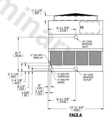
DRAWN BY: KDS NO. OF SHIPPING SECTIONS **SHIPPING** OPERATING HEAVIEST SECTION 8420 lbs+ [3820] kg+ 5550 lbs+ [2520] kg+ 15750 lbs+ [7145] kg+ WEIGHT WEIGHT WEIGHT
