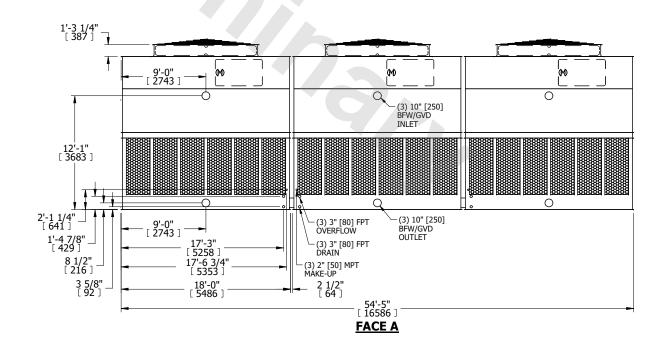
SHIPPING WEIGHT 35160 lbs+ [15950] kg+ OPERATING WEIGHT 62970 lbs+ [28565] kg+ HEAVIEST SECTION WEIGHT 7540 lbs+ [3425] kg+ NO. OF SHIPPING SECTIONS 6 DRAWN BY: KDS
