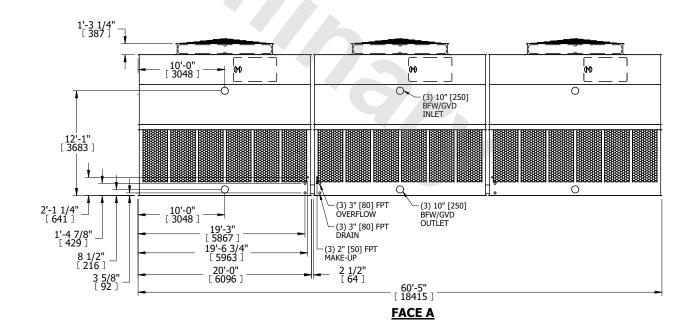
SHIPPING WEIGHT 37080 lbs+ [16820] kg+ OPERATING WEIGHT 68280 lbs+ [30975] kg+ HEAVIEST SECTION WEIGHT 7940 lbs+ [3605] kg+ NO. OF SHIPPING SECTIONS 6
