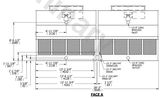
SHIPPING WEIGHT 11940 lbs+ [5420] kg+ OPERATING WEIGHT 20960 lbs+ [9510] kg+ HEAVIEST SECTION WEIGHT 3830 lbs+ [1740] kg+ NO. OF SHIPPING SECTIONS 4 DRAWN BY: JLG
