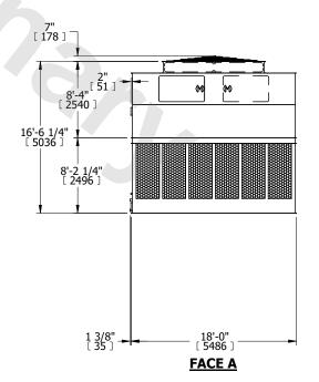
SHIPPING WEIGHT 22280 lbs+ [10110] kg+ OPERATING WEIGHT 40820 lbs+ [18520] kg+ HEAVIEST SECTION WEIGHT 6760 lbs+ [3070] kg+ NO. OF SHIPPING SECTIONS 4 DRAWN BY: KDS
