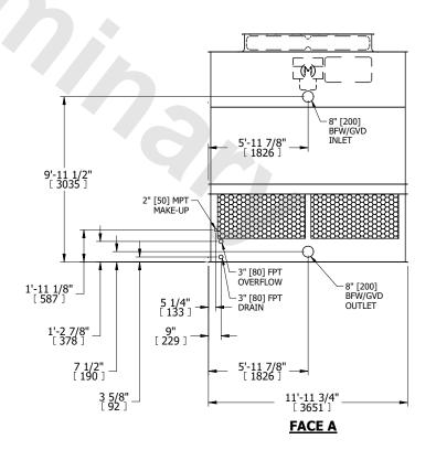
SHIPPING WEIGHT 6110 lbs+ [2775] kg+ OPERATING WEIGHT 9970 lbs+ [4525] kg+ HEAVIEST SECTION WEIGHT 4350 lbs+ [1975] kg+ NO. OF SHIPPING SECTIONS 2 DRAWN BY: JLG
