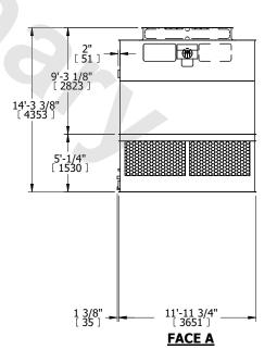
DRAWN BY: KDS NO. OF SHIPPING SECTIONS **SHIPPING** OPERATING HEAVIEST SECTION 12400 lbs+ [5625] kg+ 20120 lbs+ [9130] kg+ 4350 lbs+ [1975] kg+ WEIGHT WEIGHT WEIGHT
