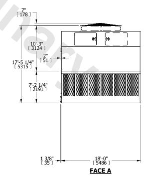
SHIPPING WEIGHT 22080 lbs+ [10020] kg+ OPERATING WEIGHT 37280 lbs+ [16910] kg+ HEAVIEST SECTION WEIGHT 7130 lbs+ [3235] kg+ NO. OF SHIPPING SECTIONS 4 DRAWN BY: KDS
