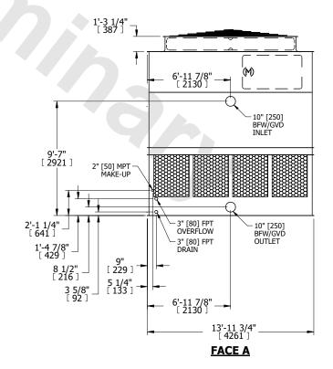
DRAWN BY: KDS NO. OF SHIPPING SECTIONS **SHIPPING** OPERATING HEAVIEST SECTION 8890 lbs+ [4035] kg+ 6020 lbs+ [2735] kg+ 16220 lbs+ [7360] kg+ WEIGHT WEIGHT WEIGHT
