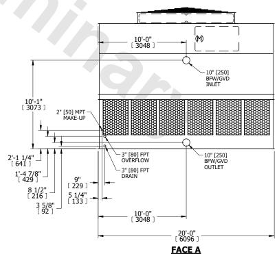
NO. OF SHIPPING SECTIONS **SHIPPING** OPERATING HEAVIEST SECTION 12100 lbs+ [5490] kg+ 22500 lbs+ [10210] kg+ 7990 lbs+ [3625] kg+ WEIGHT WEIGHT WEIGHT
