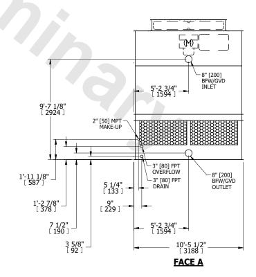
SHIPPING WEIGHT 5330 lbs+ [2420] kg+ OPERATING WEIGHT 8630 lbs+ [3915] kg+ HEAVIEST SECTION WEIGHT 3730 lbs+ [1695] kg+ NO. OF SHIPPING SECTIONS 2 DRAWN BY: JLG
