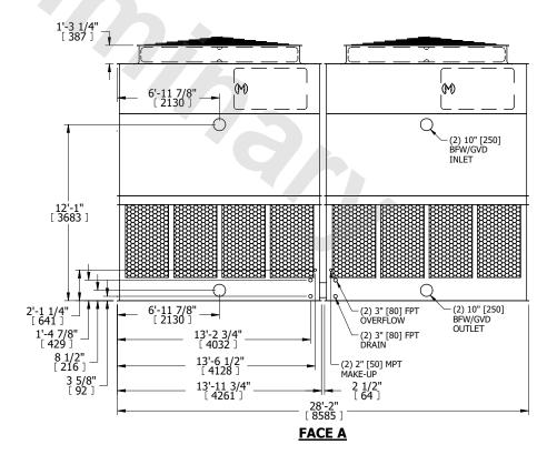
SHIPPING WEIGHT 19320 lbs+ [8765] kg+ OPERATING WEIGHT 33980 lbs+ [15415] kg+ HEAVIEST SECTION WEIGHT 6610 lbs+ [3000] kg+ NO. OF SHIPPING SECTIONS 4 DRAWN BY: KDS
