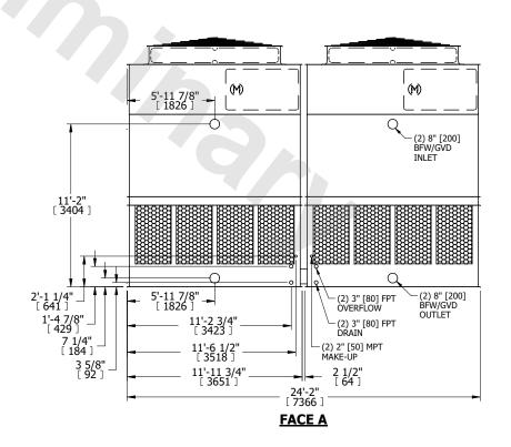
SHIPPING WEIGHT 17140 lbs+ [7775] kg+ OPERATING WEIGHT 29560 lbs+ [13410] kg+ HEAVIEST SECTION WEIGHT 6030 lbs+ [2740] kg+ NO. OF SHIPPING SECTIONS 4 DRAWN BY: KDS
