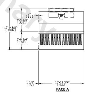
DRAWN BY: KDS NO. OF SHIPPING SECTIONS **SHIPPING** OPERATING HEAVIEST SECTION 11860 lbs+ [5380] kg+ 3790 lbs+ [1720] kg+ 20880 lbs+ [9475] kg+ WEIGHT WEIGHT WEIGHT
