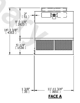
DRAWN BY: KDS NO. OF SHIPPING SECTIONS **SHIPPING** OPERATING HEAVIEST SECTION 12120 lbs+ [5500] kg+ 19840 lbs+ [9000] kg+ 4210 lbs+ [1910] kg+ WEIGHT WEIGHT WEIGHT
